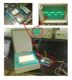
figure5. (a) Cypress Developer Board CY8CKIT-001,(b) ASIC based result for 555 implemented on PSoC,(c) A complete snap of experimental setup.
