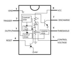
figure1: 555 Timer Block Diagram
